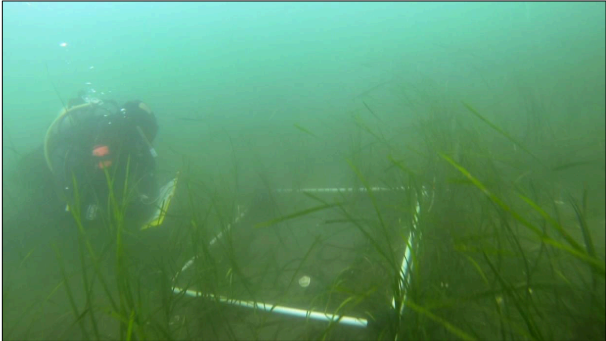
Photo 1 Quadrat (1.0 m 2 ) used to sample eelgrass and substrate conditions January 7th, 2015.
