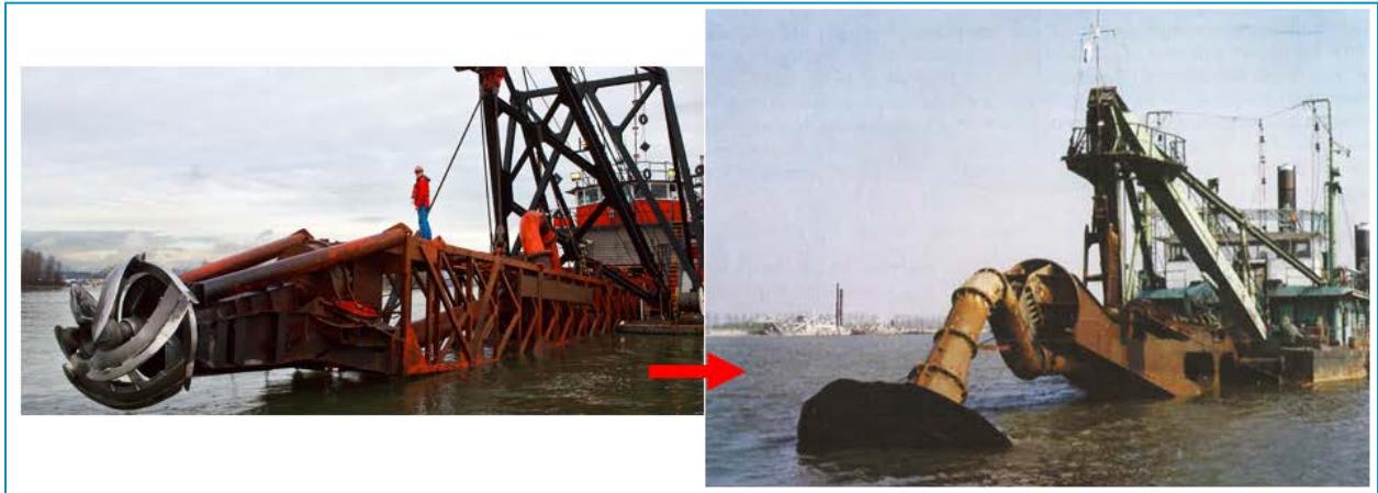
FIGURE 4-1: FRPD COLUMBIA CUTTER SUCTION DREDGE (LEFT) AND PROPOSED DIFFUSER MODIFICATION (SOURCE: FRPD)
