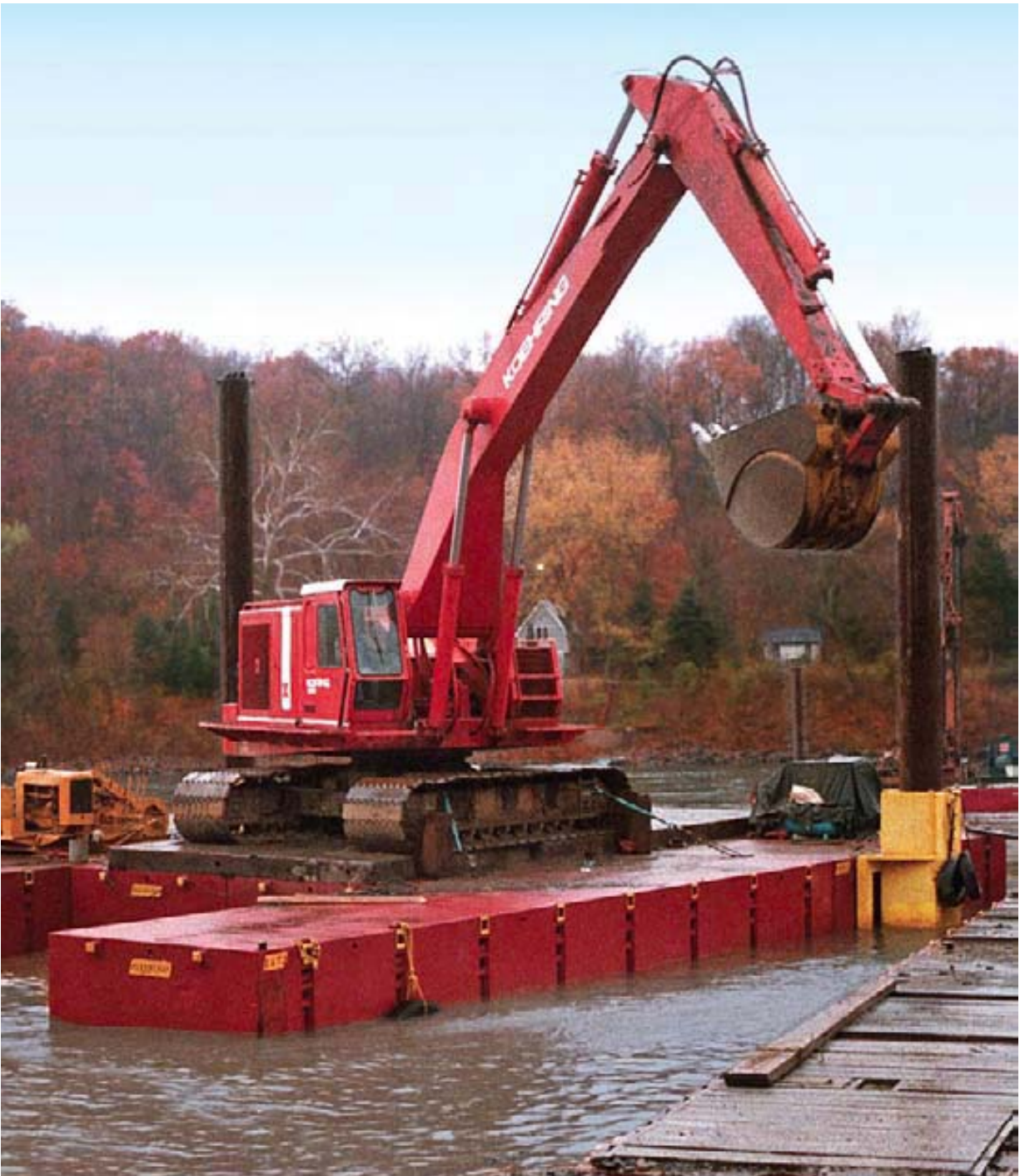
Hydraulic Excavator mounted on FlexiFloat Sectional Barges
