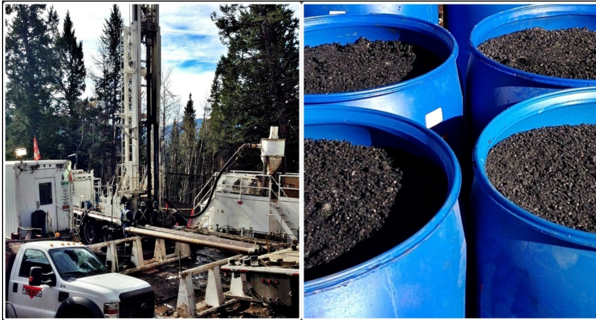
Photo B.11: Example of Reverse-Flood Drilling and Product Conducted on Grassy Mountain.
