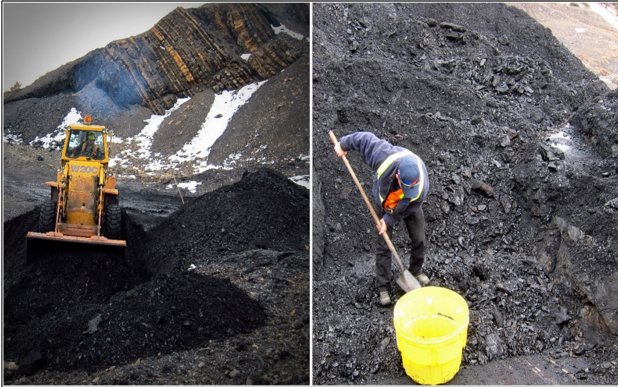
Photo B.12: Test Pit Excavation on Grassy Mountain at Seam No. 2
