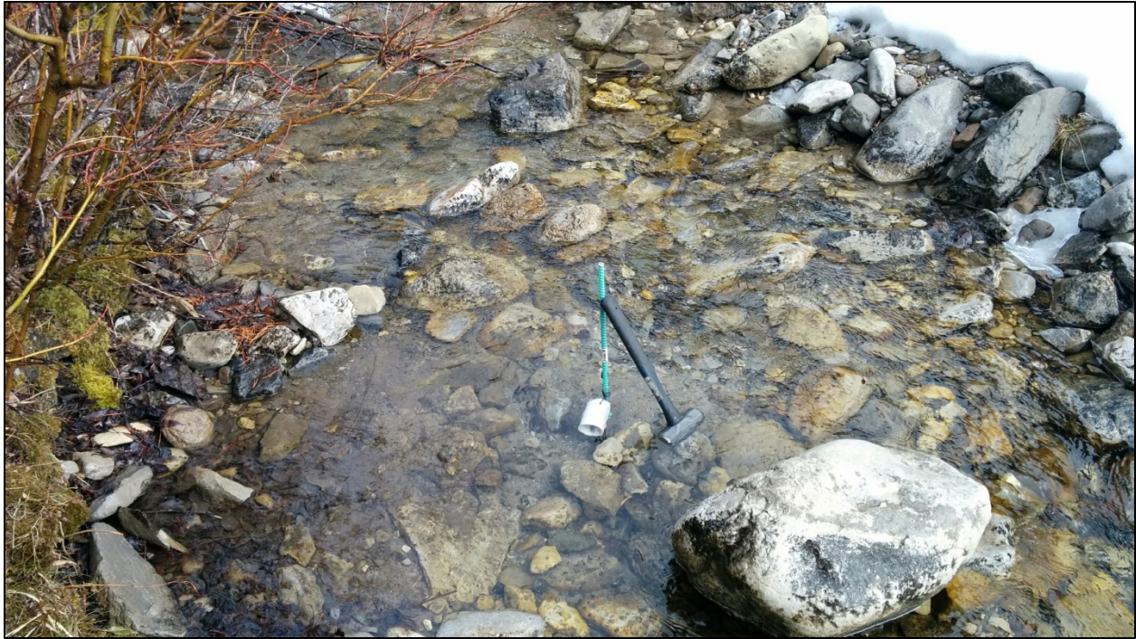
Photo 3.1 Typical installation of a water temperature logger. Hobo temperature logger is inside the white PVC pipe and attached to green rebar. Sledge hammer is for scale. Photo taken at Gold Creek Site 4 (GC-T04w) on March 21, 2016.
