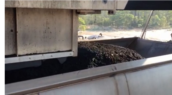
This photo illustrates the minimal drop height of coal from the TLO to the rail car. The TLO in this photo does not have external cladding. The Grassy Mountain TLO will be enclosed.
