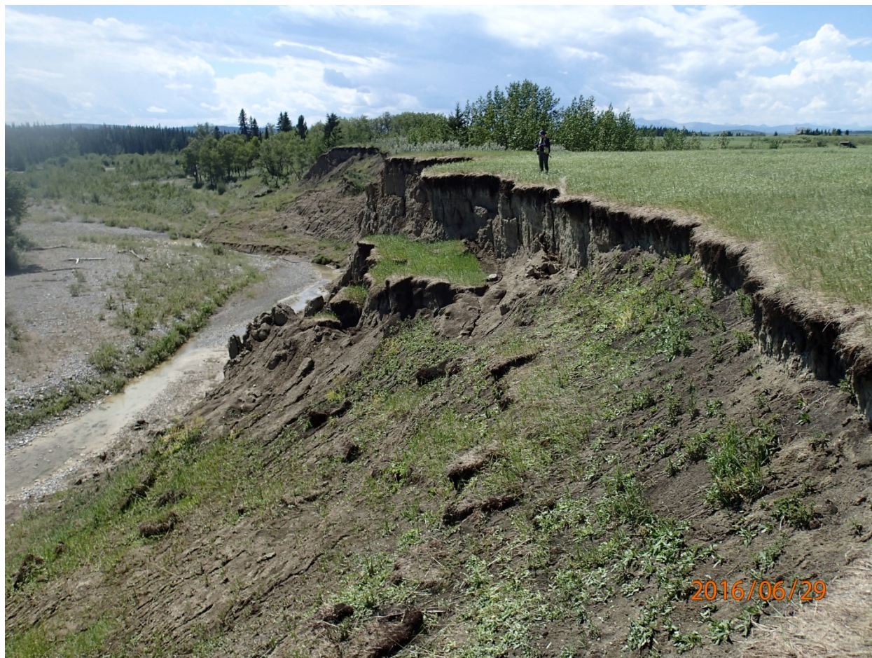
Photo 2-9 Field Photo of Surficial Material Slump in Glaciolacustrine Silt and Clay on the Elbow River Scarps
