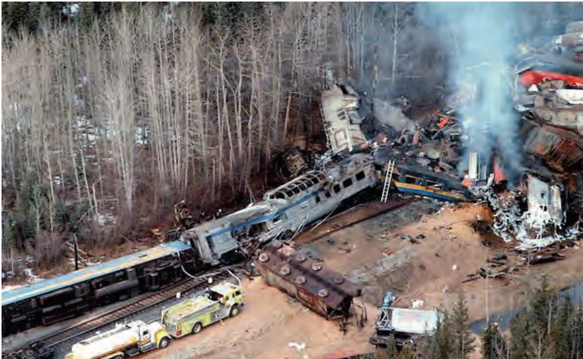
Figure K-3: Hinton collision showing the aftermath of a fire involving locomotives diesel fuel
