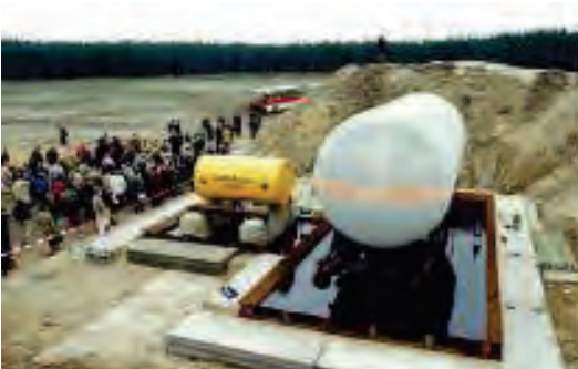
Figure 4-5: Before fire and explosion test with CASTOR THTR/AVR package placed beside LPG tank wagon
