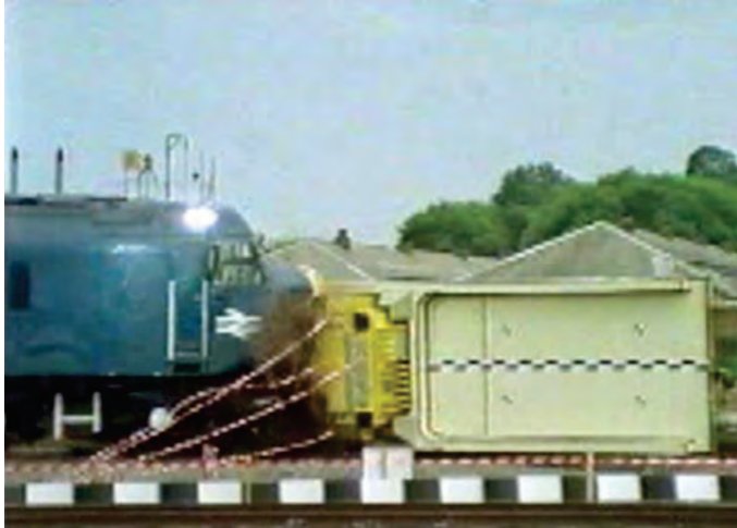
Figure 4-4: Resulting impact during Operation Smash Hit
