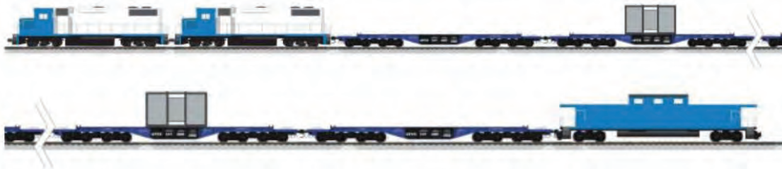
Figure 4 An illustration of the 8-axle Dry Storage Container Transportation Package Railcar
