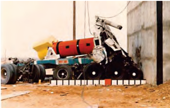
Figure 4-1: Results of truck package impact into rigid barrier
