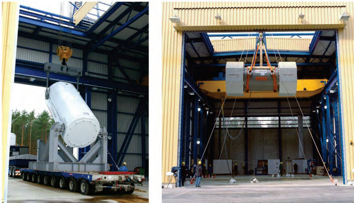
Figure E-1: Full-scale 9 m drop testing at the BAM drop test facility
