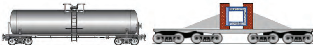
Figure M-4: Tank railcar (left) and used fuel railcar (right) – note that the DSC-TP is shipped horizontally
