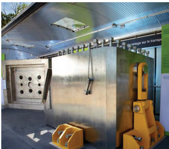
Figure 2: Used Fuel Transportation Package (UFTP)
