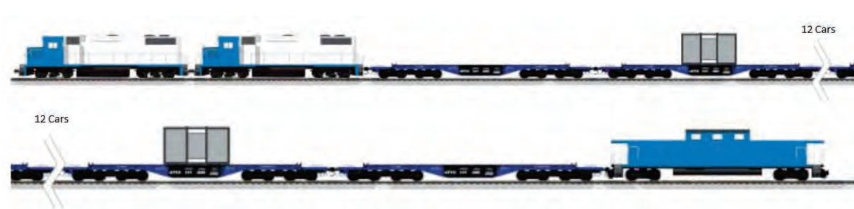
Figure 4: An illustration of the 8-axle Dry Storage Container Transportation Package Railcar
