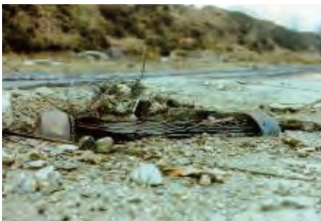
Figure 4-9: Package after drop from 200 m, penetrating concrete layer
