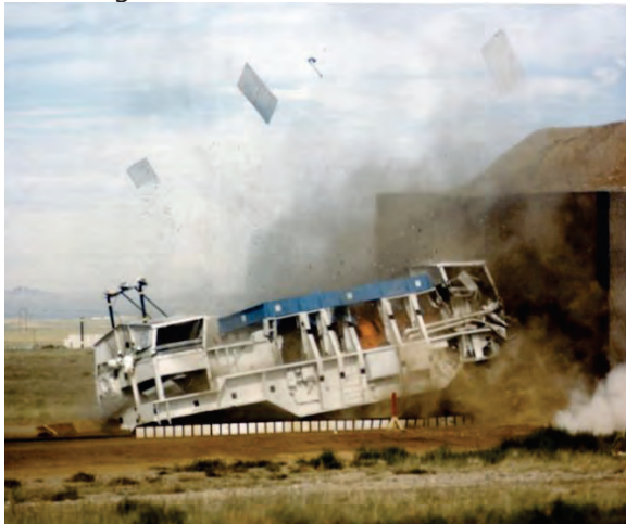
Figure 4-3: Results of rail package impact into rigid barrier
