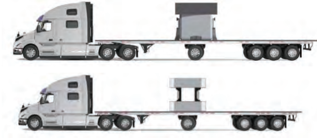
Figure 2 An Illustration of Road Conveyance with Used Fuel Transportation Package (top) and Basket Transportation Package (bottom)
