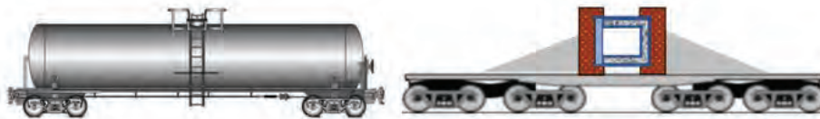
Figure J-5: Tank railcar (left) and used fuel railcar (right) – note that the DSC-TP is shipped horizontally
