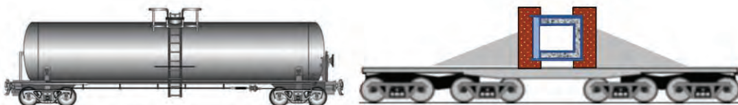
Figure K-2: Tank railcar (left) and used fuel railcar (right) – note that the DSC-TP is shipped horizontally
